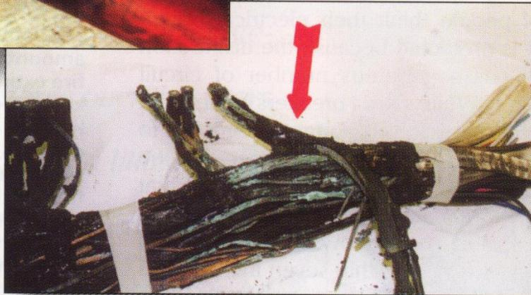
When one wire overheats, others in the same bundle can ignite. Not having proper fusing during a battery charger malfunction caused most of this boat's wiring to be damaged—a daunting repair (claim #0100202).
