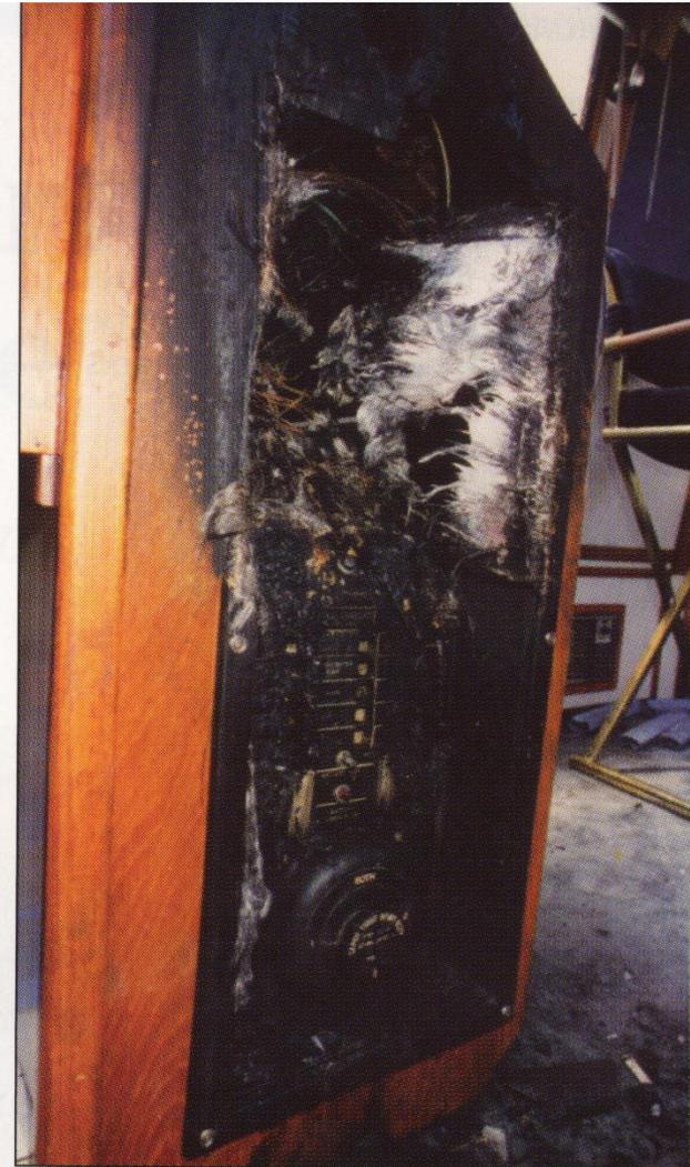
Adding a larger circuit breaker to a distribution panel without also upgrading the wiring can cause the wire to overheat inside the panel and ignite.
