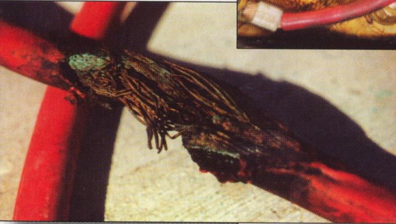
Starter cables carry a lot of electricity. This cable wasn't supported with cable clamps in the engine room and abraded against a spinning shaft. The subsequent fire began destroying the engine control cables and after the member shut down the engine, it restarted. The kill switch wiring was damaged and the engine had to be stopped by choking the air supply (Claim # 9605729).
