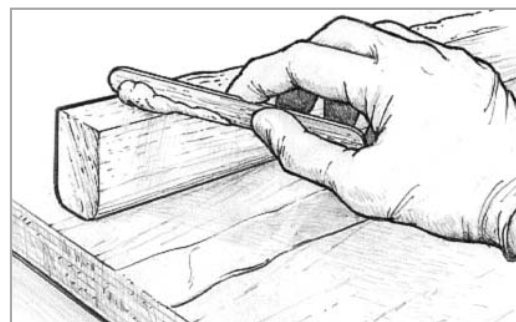
Figure 8-9 Apply thickened epoxy to one of the bonding surfaces.
