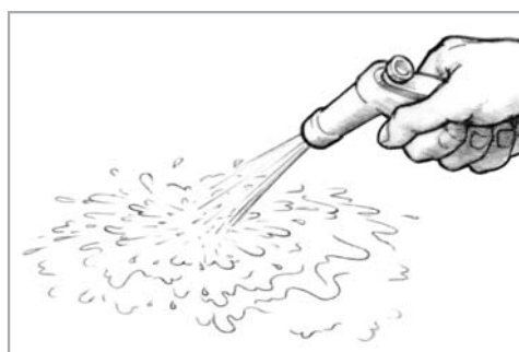
Figure 7-6 Rinse water should sheet without beading, indicating an uncontaminated surface.
