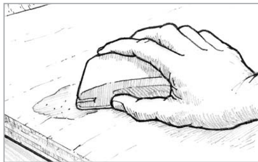
Figure 8-16 Sand the fairing material to blend with the surrounding contour.
