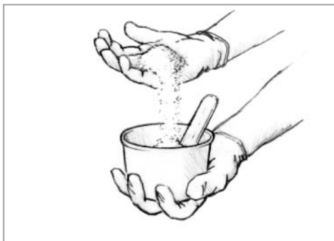
Figure 8-7 Blend in small handfuls or scoops of the appropriate filler until the desired consistency is reached.
