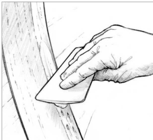
Figure 3-5 Fill the remaining voids with fairing compound.
