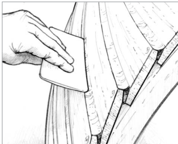
Figure 5-9 Fill the wet-out seam with thickened epoxy
